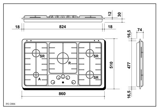
R = Rapid BurnerA = Auxiliary BurnerSR = Semirapid Burners
